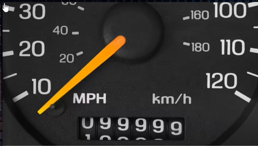
Odometers accurately count miles through a system of gears. STEPHANHOEROLD / GETTY IMAGES
